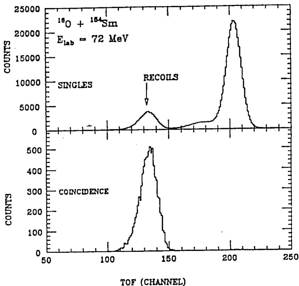
Figure 6: TOF spectra for the system  $^{16}\text{O} + ^{154}\text{Sm}$  at  $E_{\text{lab}}=72 \text{ MeV}$ , using the University of Washington electrostatic deflector, in singles (top) and coincidence (bottom) with the NaI detectors.
