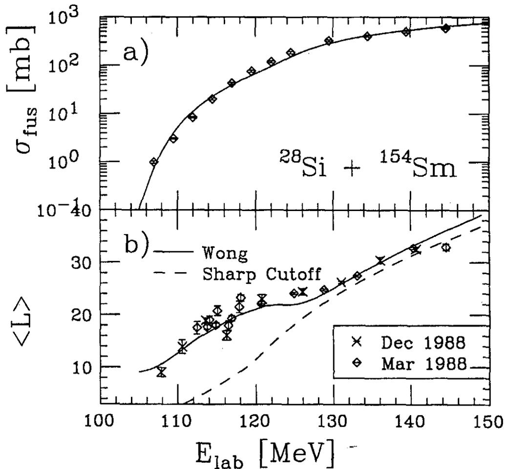
**Figure 7:** Preliminary results of  $\langle \ell \rangle$  obtained from  $M_\gamma$  measurements using an electrostatic deflector. The solid line are Wong model predictions, using parameters that also fit the fusion excitation function for this system (see fig. 5). From ref.[35].
