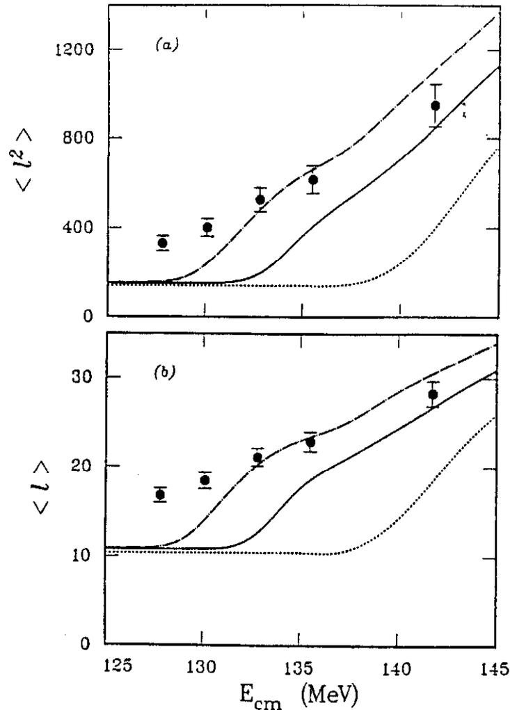
**Figure 9:** Results of  $\langle \ell \rangle$  and  $\langle \ell^2 \rangle$  for the system  $^{64}\text{Ni} + ^{100}\text{Mo}$ . The dotted lines single barrier penetration calculation. The full curves are coupled-channel calculations with established coupling parameters. The dot-dash curve are the result of increasing the coupling parameters by 50%. From ref.[22].
