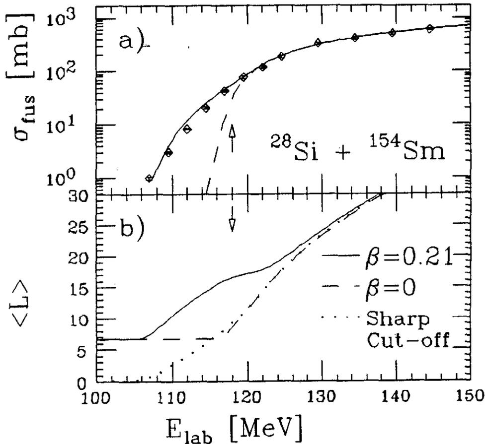
**Figure 5:** Illustration of the effect of deformation on the  $\sigma_{fus}$  and  $\langle \ell \rangle$ . The introducing of ZPM or coupling to other channels produce qualitatively similar results [20, 2]. These effects can also be simulated with a fluctuating barrier. Note that below the lowest barrier thus generated, the same saturation value is obtained. The experimental result are from ref.[35]
